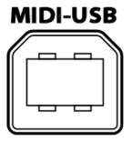
An additional Type-B USB 2.0 port is present at the back side of the Mojo Desktop that provides Class-compliant USB-MIDI IN/OUT connection to your computer. Use this port to connect the Mojo Desktop to your computer software. No drivers are needed for Windows, OS X and Linux.
