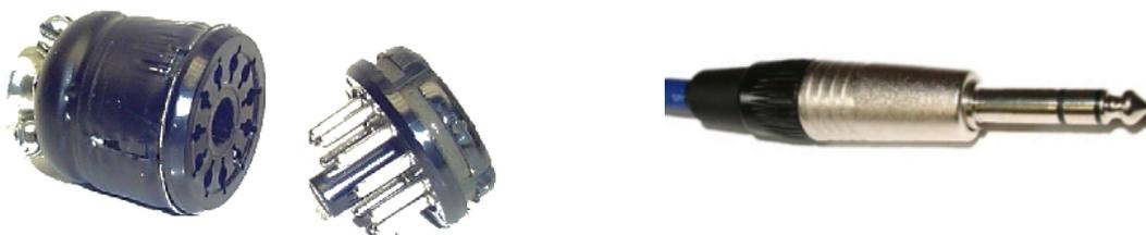
The most common connectors used in modern rotary speakers are the 11-pin relay type connector and the TRS connectors. The following table shows how to connect the MIDI board to the 11 pin connector, which is the only known standard still used today for rotary speakers.
