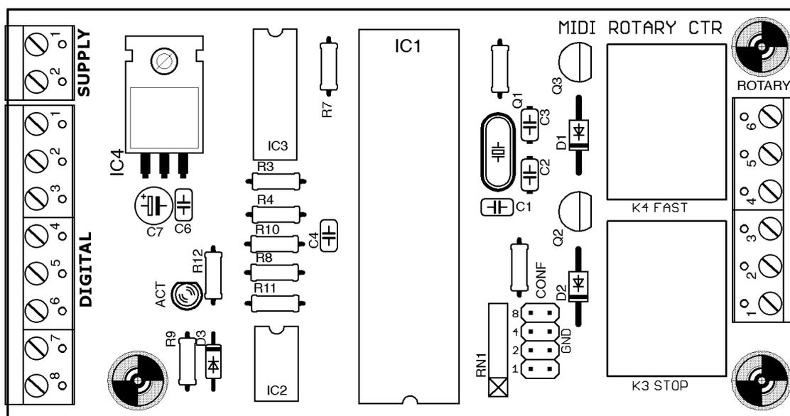
The connections are offered under the form of screw terminal blocks, that are sockets into which you can insert a wire and lock it with a screwdriver. This way you don't have to solder anything. Sockets are on the two sides of the board. As you can see from the picture above, on the left side you have, from top to bottom:
