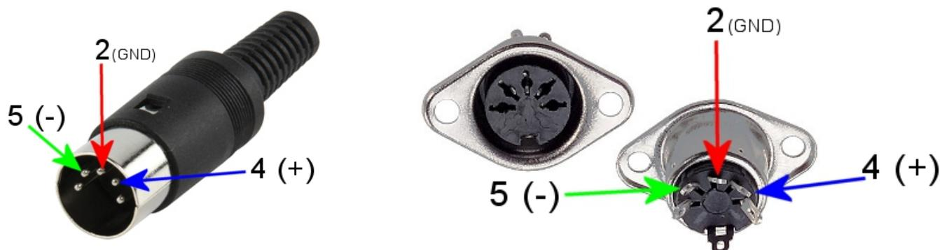
The above image shows the pinout of both the male DIN5 cable connector and the female DIN5 panel connector. The center pin is connected to ground and is only used for the MIDI output ports (which include the THRU port), while the MIDI input only use the pins 4 and 5. Pay attention not to swap these pins or your MIDI connection won't work.
