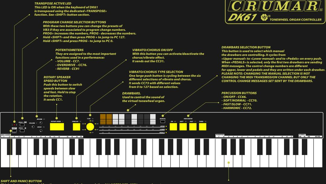
This is a button with special functions: as soon as it is depressed, the «ALL NOTES OFF» MIDI message is sent. Hold it down in combination with some other buttons and keys of DK61 to perform specific operations. These are highlighted in the panel.
