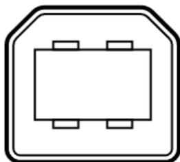
An additional Type-B USB 2.0 port is present at the back side of the Mojo 61 that provides Class-compliant USB-MIDI IN/OUT connection to your computer. Use this port to connect the Mojo 61 to your computer software. No drivers are needed for Windows, OS X and Linux. Use this port to connect the USB cable for USB online editor.
