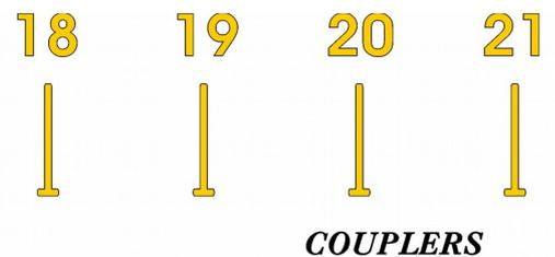
Let's make an example: play the center C-note, now push button n. 18, this will activate the “SUB OCTAVE” coupler and you'll hear the lower C adding to the sound; now push button n. 19 that will activate the “OCTAVE” coupler, so that the higher C will also add to the sound; lastly, button n. 20 enables the “CANCEL UNISON” which will cancel the center note, i.e. the note that you are actually playing, leaving only the lower C and the higher C.
